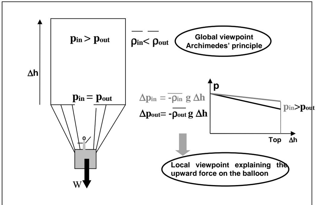
Figure 7. Some elements needed to understand how a hot air balloon stays in the air. W: weight of the system (basket+load+balloon). The unlikely cylindrical shape is intended to facilitate the understanding of how a resulting upward force is linked to a difference between internal and external pressure (Viennot 2006)
